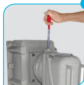
Locking the plug in the socket closes the pilots and connects the main circuit.
